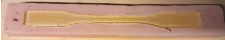
Fig. 3. EN ISO 527-2:2012 1B Specimen with 0% OSA filler in the silicone mould curing
